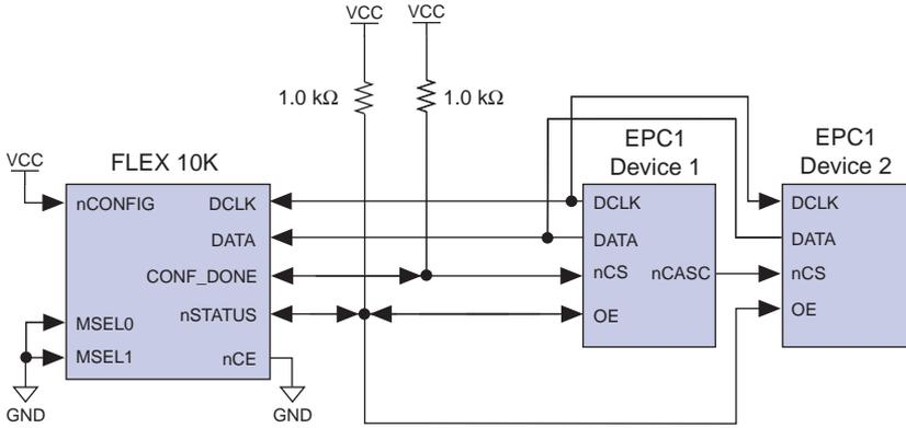
Figure 6 shows two FLEX 10K devices configured with two EPC1 devices.
